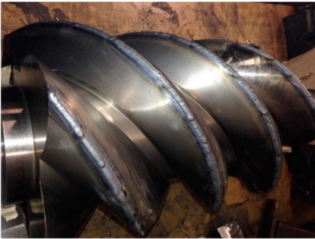
Rotor tips welded up and ready for first stage of cylindrical grinding.
